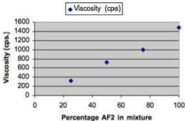
Graph showing how the viscosity of AF2 solution is influenced by adding AF1 solution
