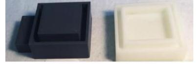
2. Load TEM grids into slits of Grid support plate with fine forceps at identified locations then slowly unclip from the Modified Hiraoka plate holder.
